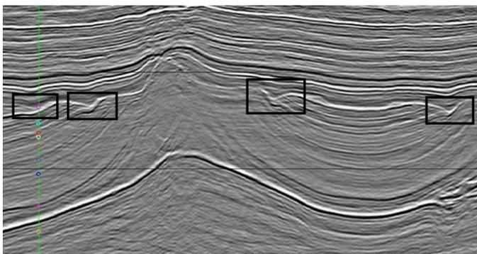
Fig. 1 Subrosional sinks of Triassic evaporites below the Late Cimmerian unconformity (c. Base Lower Cretaceous) near the German border in the NL part of the North Sea.
