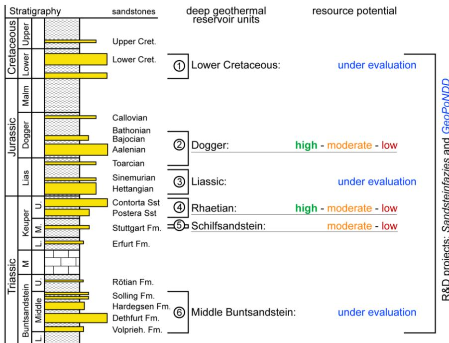
Fig. 1: Mesozoic sandstones and deep geothermal reservoirs of the North German Basin.
