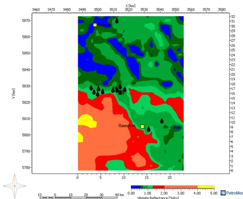
Fig. 1 - Thermal maturity map of the Posidonia Shale for parts of the LSB, Gifhorn Trough and Pompeckj Block showing the location of the analysed oil samples, modified after Bruns et al. (2014).
