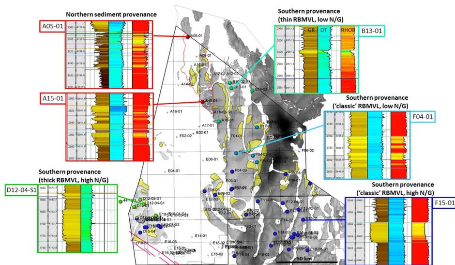
Fig. 5: Regional reservoir architecture – typical well log response for different types of Volprieausen sandstone (RBMVL). Study area is outlined in solid black, yellow polygons indicate Triassic leads.
