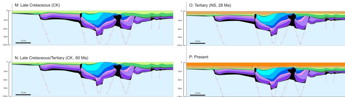
Fig. 4: Depth converted and structurally restored models of the seismic section shown in Fig. 1. These models show the Late Cretaceous to Present configurations, which represent four (4) out of in total sixteen (16) restoration steps presented in this study.
