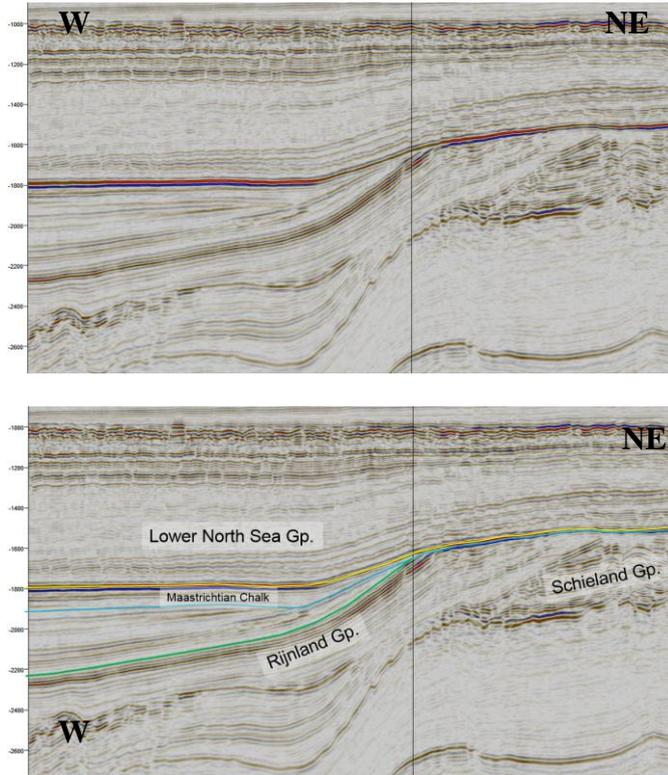
Seismic section Dutch offshore blocks L1 and L2, western flank of inverted Central Graben. Un-interpreted and interpreted section. Thin Maastrichtian Chalk is present over inverted Central Graben. Yellow: Top (Maastrichtian) Chalk, Blue: Sub-Hercynian Unconformity (note phase change) and Green: Base Texel Chalk.
