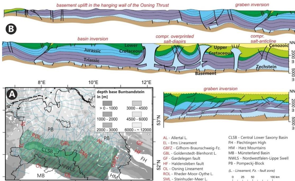
Fig. 1: A.) Structural overview map of the LSB and surrounding areas. Additionally, the geological 2D-profiles of the GTA are plotted; B.) Exemplary geological profiles redrawn after the GTA. Typical structures with a Late Cretaceous contractional overprint within and along the borders of the LSB are highlighted.
