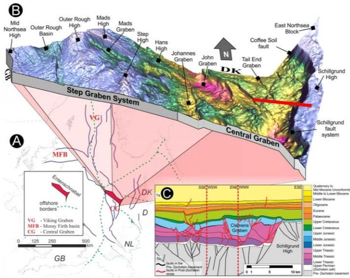
Fig. 1: a) Overview map of the North Sea region with location of the study area (Entenschnabel) and the main graben systems; b) 3D view of the Top Pre-Zechstein (blue to green colours indicate structural highs; pink to yellow colours show structural lows); c) cross-section with structural interpretation across the Schillgrund fault; line of section is highlighted as red line in b).
