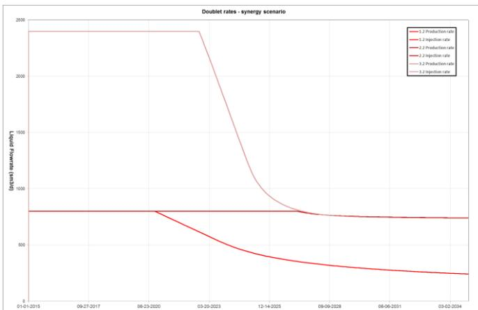
Fig. 3: During a synergy scenario the doublet rates cannot be maintained due to the declining reservoir pressure.
