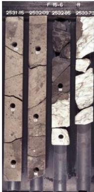
Fig. 1 The base of the caprock succession of well F15-06. Dark mudstones with angular clasts overlie Zechstein evaporates and grade upwards into sandstones with matrix supported clasts.
