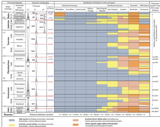
Fig. 1: Stratigraphic column showing Lower and Middle Jurassic ammonite zones together with T-R cycles and the levels of paleo biofacies maps constructed in this study. Table compiled from data by Zimmermann et al. (2015) and Barth et al. (in review).
