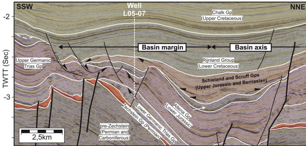
Fig. 1. Interpreted seismic section in the Terschelling Basin (block L5) showing the southern basin margin. Black arrows show truncation and stratal onlaps.
