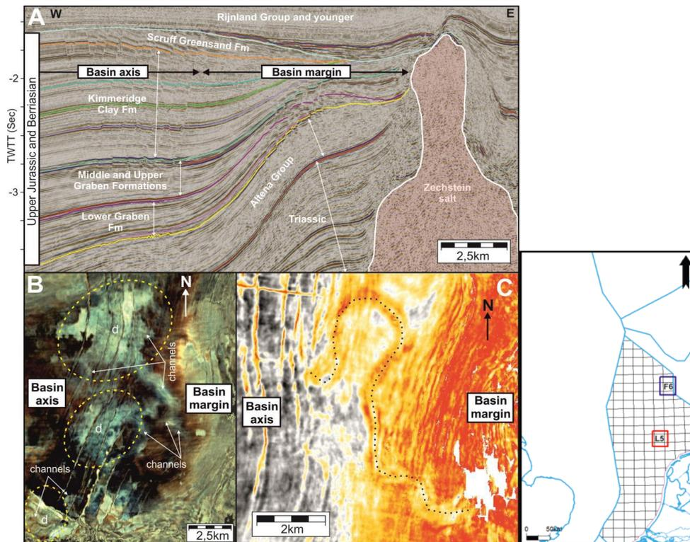
Fig. 2. Interpreted seismic section in the Dutch Central Graben (block F6) (A), spectral decomposition of the upper part of the Upper Graben Formation (B) and sweetness attribute of the upper part of the Lower Graben Formation (C) along the eastern margin of the Dutch Central Graben (block F06). Small laterally offset deltas (d) and associated channels are observed in Fig. 2B.
