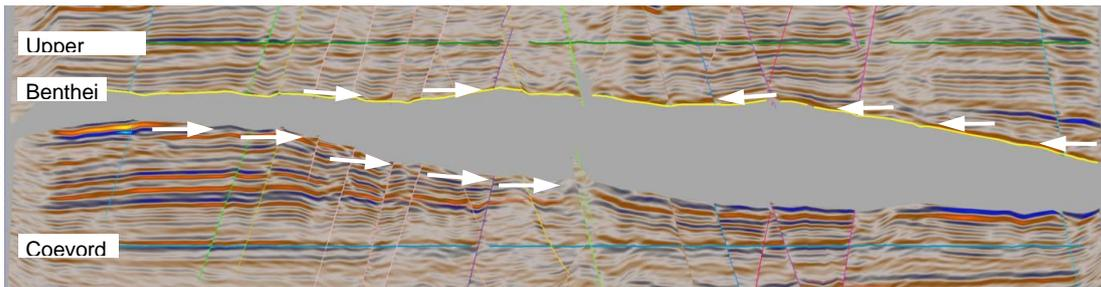
Fig. 4: Stratigraphic display with unconformity gap at base-Bentheim unconformity. Unfolded on horizons above and below the unconformity. White arrows for seismic reflection terminations (approx.).
