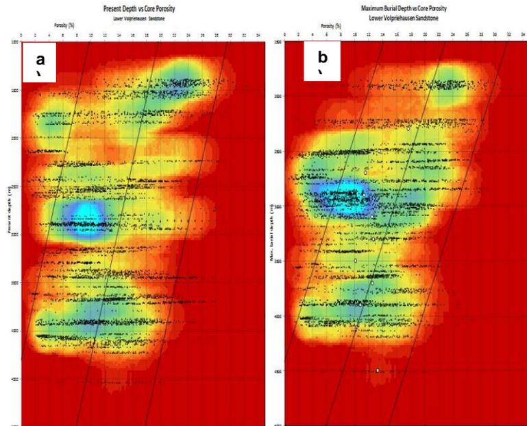
Fig. 2: Porosity - depth graph of the Lower Volpriehausen Sst Mbr. (a) core plug porosity values versus present day depth and (b).maximum burial depth. The open circles are the 200m depth interval averages
