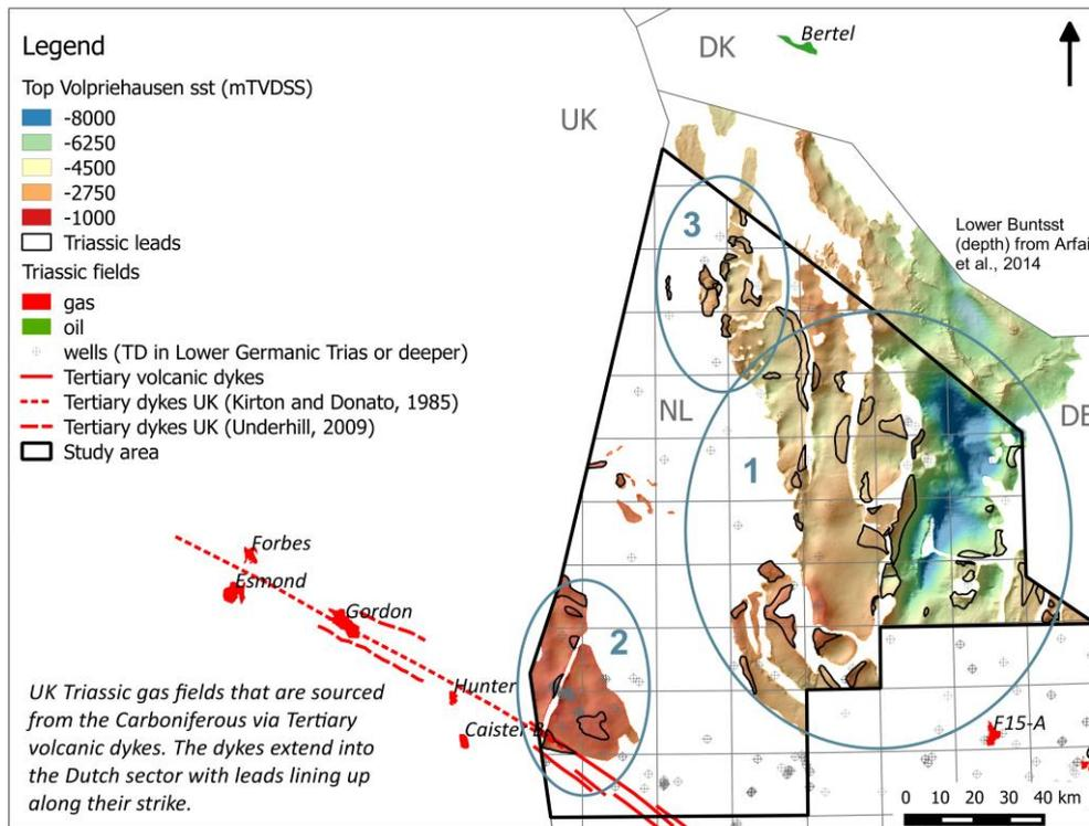
Fig. 6: Top Volpriehausen sandstone depth map in the study area. The identified leads are separated in three types (1- 'classic'; 2- sourced via volcanic dykes, 3- northern reservoir provenance).
