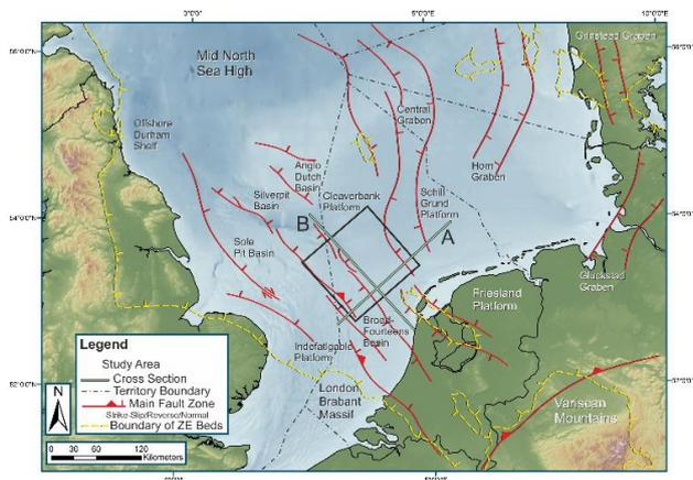
Structural and seismic-stratigraphic analysis of a basin-scale 3D seismic dataset allowed: (1) refinement of the existing regional tectonostratigraphic models, specifically for the Broad Fourteen Basin with its complex thick-skinned and thin-skinned structural history. (2) Correlation of salt tectonic processes with major regional tectonic events. (3) Assessing the hydrocarbon potential of supra-salt plays.
