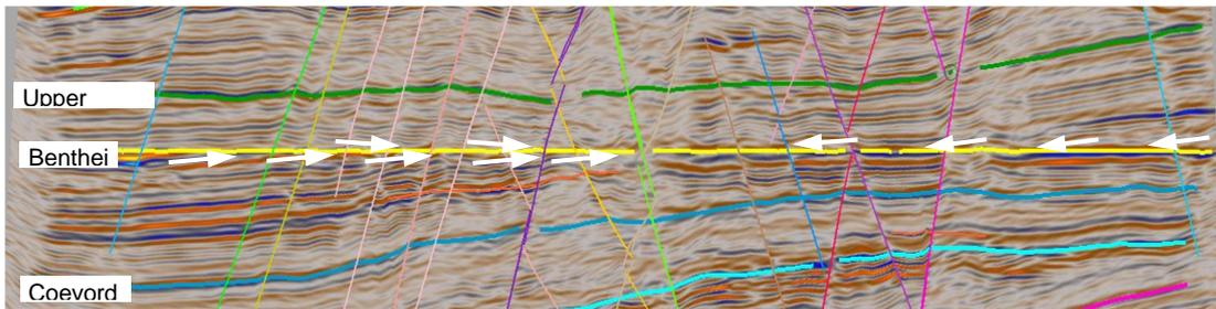
Fig. 3: Structural display unfolded on base-Bentheim unconformity. White arrows for seismic reflection terminations (approx.).
