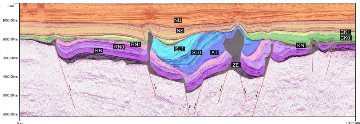
Fig. 2: The interpreted seismic section (TWT) that was structurally restored in this study, transecting the Dutch Central Graben and Step Graben and the margins of the Elbow Spit Platform and Schill Grund Platform. The location of this section is shown on Fig. 2. Tertiary North Sea group (NS), Cretaceous Chalk group (CK), Jurassic Schieland group (SL) and Altona group (AT), Upper Germanic Trias group (RN) and Lower Germanic Trias group (RB), Permian Zechstein group including the salt (ZE)
