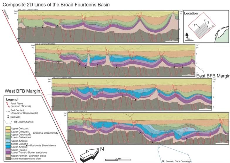
Fig.2: Composite parallel fence diagram displaying the spatial evolution of the Broad Fourteens Basin, Southern North Sea, in the SW-NE orientation. (Red line: perimeter of study area, Blue Line: Perimeter of 3D seismic coverage)
