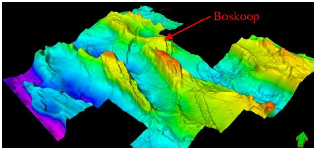
Fig. 1: Structure of the Boskoop field and surrounding area. Surface from seismic interpretation, base Alena.
