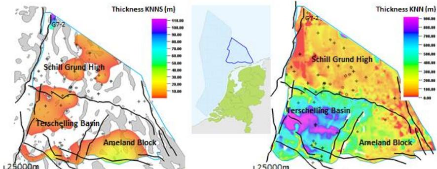
Fig. 1a: Vlieland Sandstone thickness, based on well data only<sup>1</sup>. Grey outlines are salt structures. (\* The thickness is often below seismic resolution and therefore very difficult to pick on seismic).
