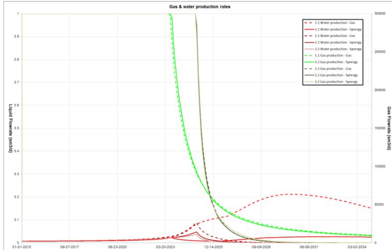
Fig. 2: Gas and water production rates of the gas well. Case 1: Boskoop properties, case 2: high permeability, case 3: high permeability and higher doublet rate.
