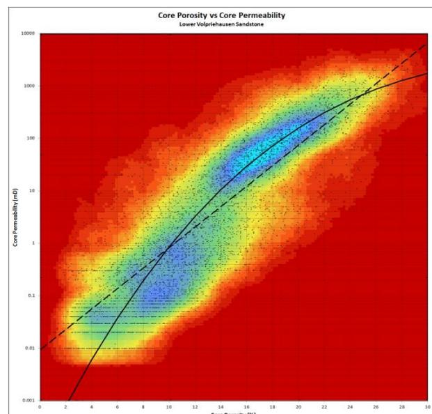
Fig. 1: Permeability vs porosity cross plot of core plug measurements of the Lower Volpriehausen Sst.
