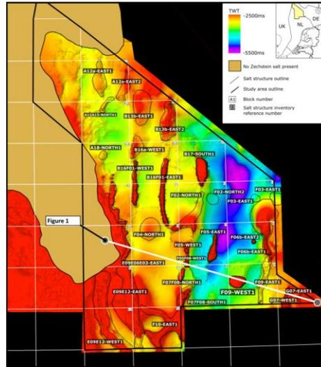
Fig. 3: Top Zechstein time structure (ms) map; all 30 identified salt structures are outlined (dotted black outlines) and referenced to the salt structure inventory, which was compiled in this study.
