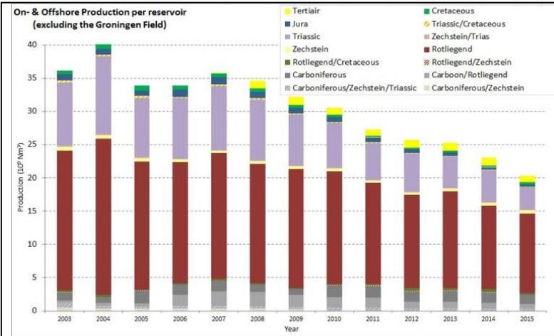
Fig. 1: Dutch yearly offshore gas production volumes by reservoir. (based on MEA 2015)
