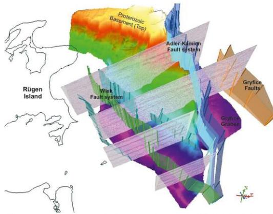
Fig. 2: 3D view of the study area (Gridded horizon: top of Proterozoic, Fault Systems: AKFS (blue), WFS (green) and Gryfice Faults (orange)).
